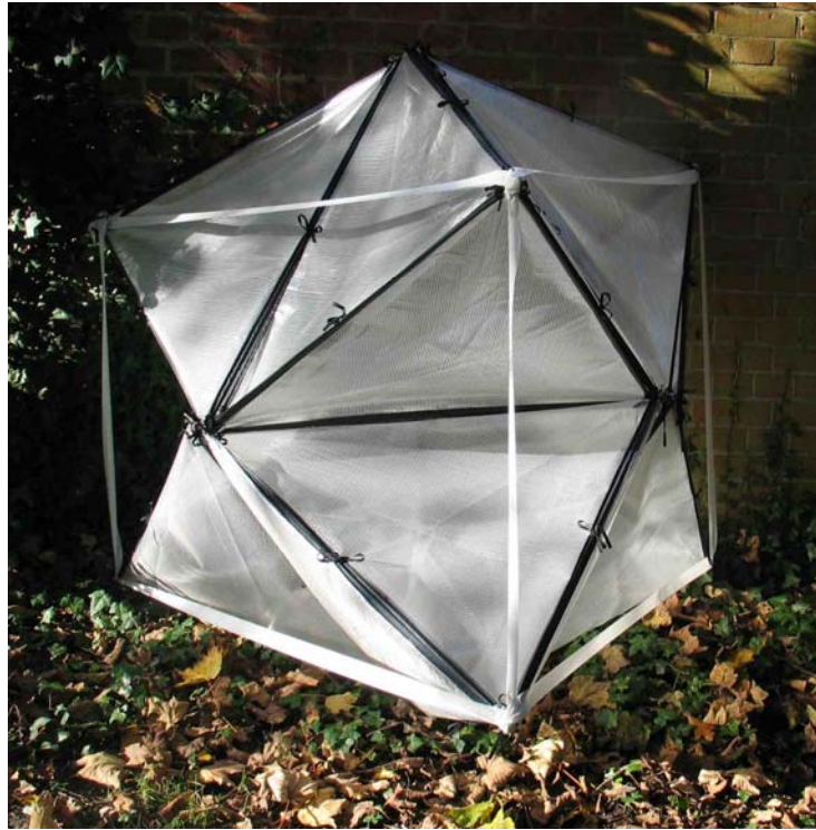
Figure 8 All apexes connected by tape
