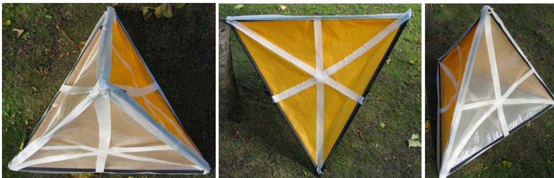
Figure 9 Taping round all reflection planes on a tetrahedron (the middle image is not completely taped)
